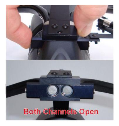
When storing the illuminator in the carry case, always return the shutter to this center position.
