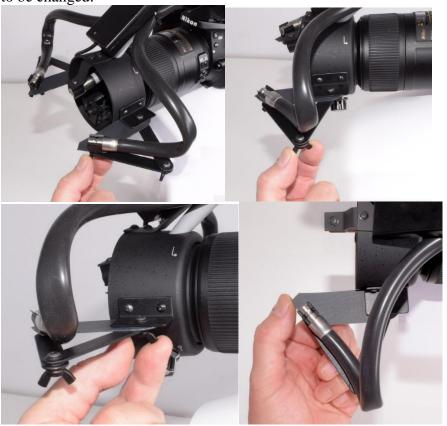
3. After loosening the 3 wingnuts, pull the output end of the lightguide away from the Alignment
