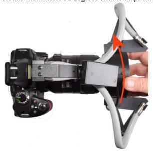
9. Rotate focus light power control clockwise to switch it on:
