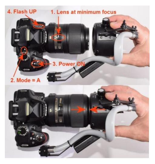
8. Rotate Illuminator 90 degrees until it snaps into place at 12:00 position:
