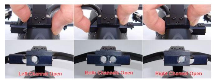
2. For "flat" or uniform illumination, use the **Both Channels Open** position. This is setting is when the shutter is in the center position:
