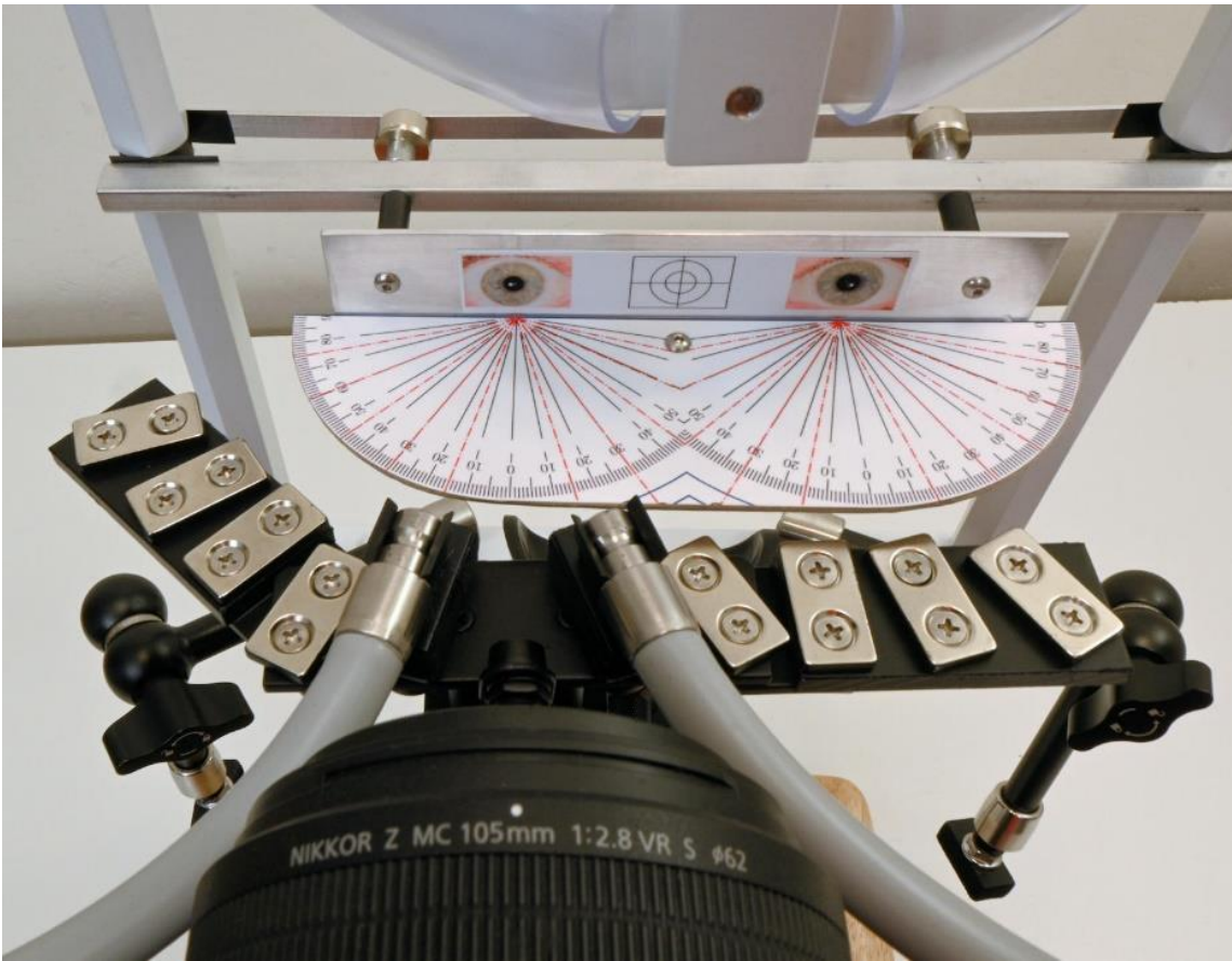
When photographing an iris, the illuminator arm is folded out on the lateral side of the eye, which allows the light source to present a similar amount of light to the iris at any angle. This simplifies exposure and saves time.
