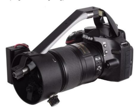
This is the simple, easy-to-use central lighting camera. It is ideal for both human and animal iris imaging. The light is positioned at 13 degrees from the axis to avoid shadows and other artifacts, and to keep the reflection off cornea in the pupil area.
